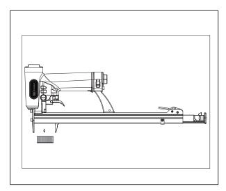
**1.** With magazine fully open, insert fasteners. Set staples strip into the magazine and keep the points of fasteners in contact with groove.
