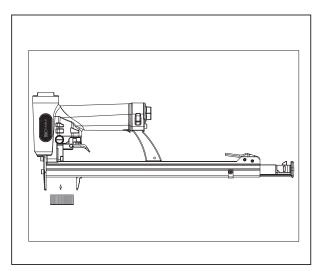
**1.** With magazine fully open, insert fasteners. Set nail strip into the magazine and keep the points of nails in contact with groove.
